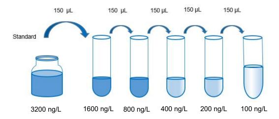
**Note**: If samples generate values higher than the highest standard, please dilute the samples with Sample Diluent and repeat the assay.
